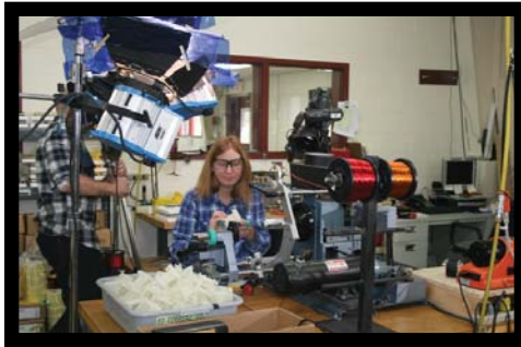
Tunie Mitchell showing the first stages of winding a transformer
